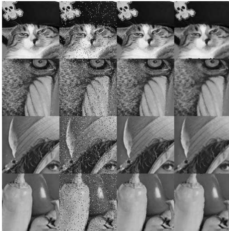
Fig. 5. Results of evolution for the salt and pepper noise removal problem. Each tile shows a crop (128x128 pixels) of the input images. The first column of images shows the original image. The second column shows the image with added noise. The third column shows the result of noise removal using an evolved filter. The final column shows the effect of apply a median filter to the noisy image.
