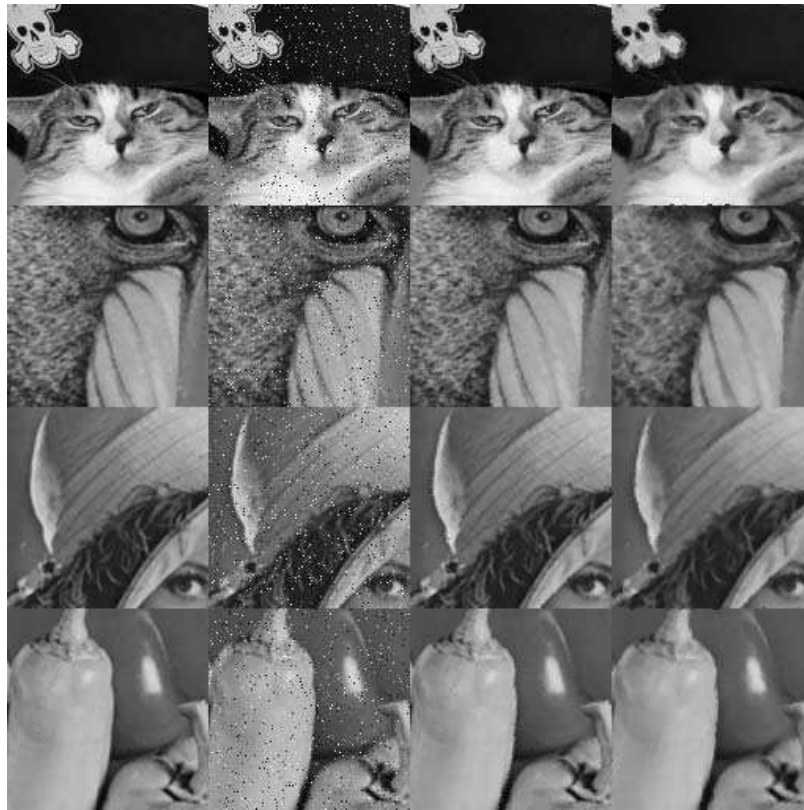
Fig. 4. Results of evolution for the noise problem. Each tile shows a crop (128x128 pixels) of the input images. The first column of images shows the original image. The second column shows the image with added noise. The third column shows the result of noise removal using an evolved filter. The final column shows the effect of apply a median filter to the noisy image.
